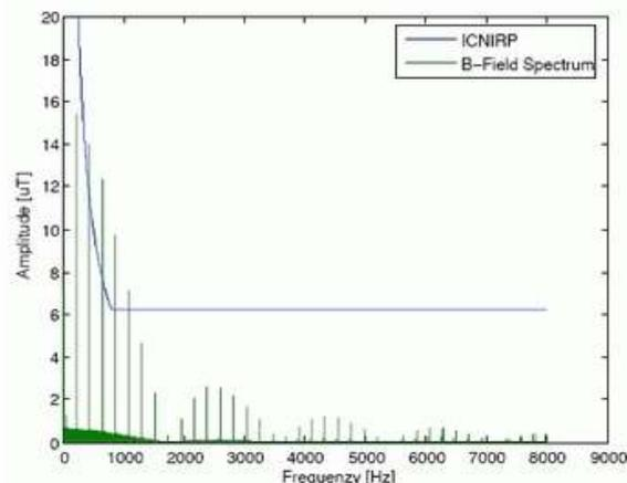
Figure 3: Magnetic field of a GSM mobile phone as a function of frequency and the frequency-dependent ICNIRP exposure limit. Evidence of values many times higher than 217 Hz. Source: [6]
