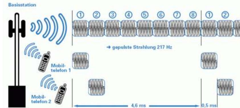
Figure 1: GSM network diagram: The mobile phone only transmits for 1/8 of the call time, which results in a pulsed radiation of 217 Hz.
