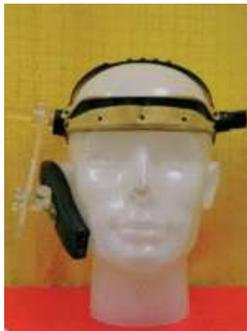
Figure 2: Head phantom for determining the specific absorption rate. Photo source: [2]
